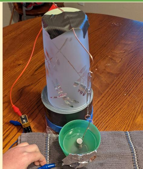
**My completed Faraday motor. The magnet pile is in the cup. The copper wire dangles around the pile. Electricity connects because the alligator clips are metal, and the edge of the cup is metal. The only part not connected with metal is the saltwater. (This picture was actually the second try later, when I switched out saltwater to try again. This cup is green. By this time, it only worked a few seconds.**
