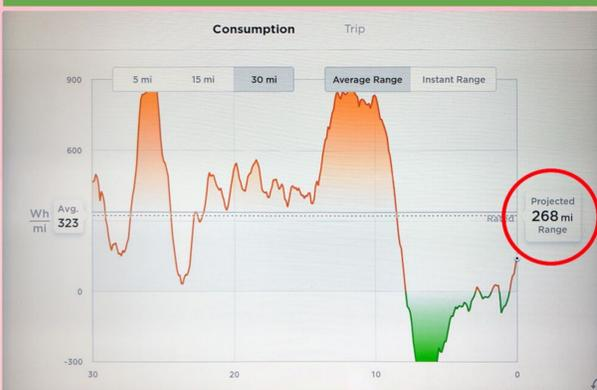
The pictures shows energy flow in an electrical car. In the orange region the motor is using energy. In the green region the battery is being charged when the car decelerates.
